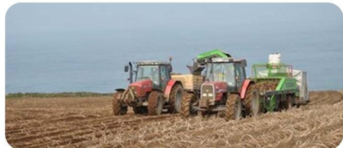
The potato harvester 'lifts' the potatoes out of the ground. It pushes them through the harvester on a belt shaking them as they go to shake any soil off. It then drops them into a trailer.
