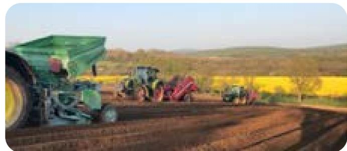
Potato seeds are planted in the soil. The machine drops the seed tubers at regular intervals in furrows and covers them with the help of two discs.
