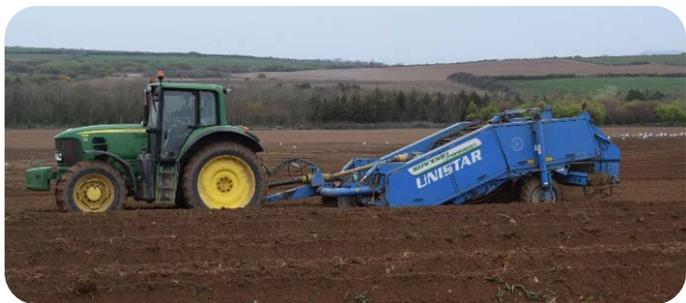
Stone separators take out any big stones as well as break up big clumps of soil. Harvesters do not know the difference between stones and potatoes.
